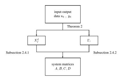
**Figure 2.4** An overview of the deterministic subspace identification procedure. Through the main Theorem 2 the state sequence  $X_f^d$  and the extended observability matrix  $\Gamma_i$  are determined. The system matrices are then extracted using any of the two algorithms described in Sections 2.4.1 or 2.4.2.
