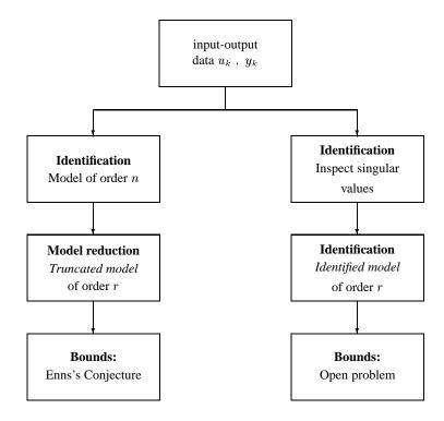
**Figure 5.3** The left hand side of the Figure illustrates how first an *n*th order model is obtained through identification, after which it is truncated to obtain the *truncated* lower order model. The right hand side illustrates how the reduction can be done in the identification step. This leads to the *identified* lower order model.
