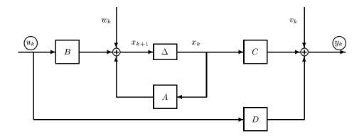
**Figure 4.2** A linear time-invariant combined deterministic-stochastic system with inputs  $u_k$ , outputs  $y_k$  and states  $x_k$ , described by the matrices A, B, C, D and the covariance matrices Q, S, R. The symbol  $\Delta$  represents a delay. In the combined identification problem, the input and output signals are measured. The state is unknown, but will be determined as an intermediate result of the subspace identification algorithms.
