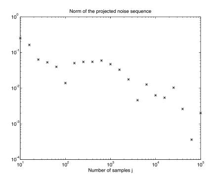
**Figure 1.11** Norm of the projected noise sequence e/u, where e and u are vectors with j samples. The norm goes to zero with a factor  $1/\sqrt{j}$  as can be seen from the Figure. When j is large enough and e is a zero mean white noise sequence, e and u can be considered perpendicular to each other ( $\parallel e/u \parallel = 0$ ). This illustrates why subspace algorithms work well, even in the presence of noise (when a large number of samples is available).
