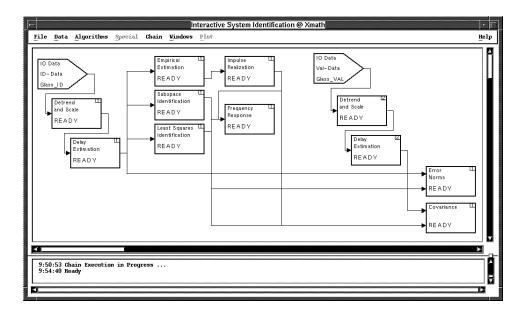
**Figure 6.9 ISID** chain representing the identification of the industrial glass-tube manufacturing process. Each block represents an algorithm. The blocks to the left are the input-output data and preprocessing blocks, followed by the identification blocks. To the right, we also see some validation blocks. Behind each block there is an algorithm window that visualizes the algorithm specific data and allows for adjustment of the parameters.
