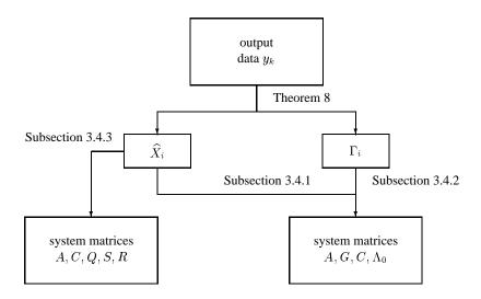
Figure 3.8 An overview of the stochastic subspace identification procedure. Through the main Theorem 8 the state sequence  $\widehat{X}_i$  and the extended observability matrix  $\Gamma_i$  are determined. The system matrices are then extracted using any of the three algorithms described in Sections 3.4.1, 3.4.2 or 3.4.3.
