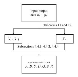
Figure 4.4 An overview of the combined deterministic-stochastic subspace identification procedure. Through the Theorems 11 and 12 the state sequence  $\widehat{X}_i$  ( $\widetilde{X}_i$ ) and the extended observability matrix  $\Gamma_i$  are determined. The system matrices are then extracted using any of the three algorithms described in Sections 4.4.1, 4.4.2 and 4.4.4.
