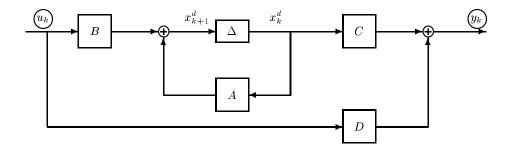
Figure 2.2 A linear time-invariant deterministic system with inputs  $y_k$ , outputs  $y_k$  and states  $x_k^d$ , described by four matrices A,B,C and D. The symbol  $\Delta$  represents a delay. Note the inherent feedback via the matrix A (representing the dynamics). In the deterministic identification problem, the circled signals (input  $y_k$  and output  $y_k$ ) are known. The state is unknown, but will be determined as an intermediate result in the subspace identification algorithms.
