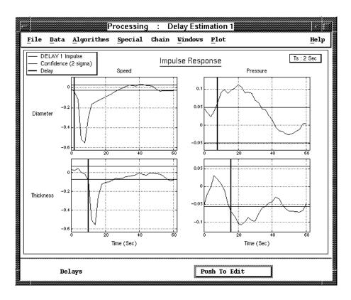
**Figure 6.10** The **ISID** algorithm window for the delay estimation algorithm. The delays are indicated by the vertical lines. They can be changed by clicking on the vertical lines and dragging them to the desired value i.e. the intersection of the impulse response and the confidence bounds (horizontal lines). This contrasts with the Command-line User Interface where the user had to read the intersecting point from the scales.
