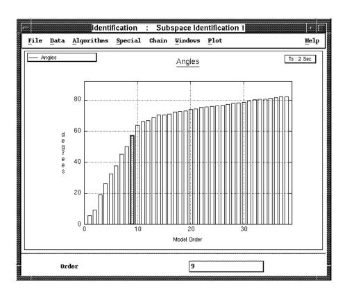
**Figure 6.11** The algorithm window behind the subspace identification algorithm. The plot displays the principal angles (algorithm of Figure 4.8 with  $W_{\rm I} = \Phi^{-1/2}_{[Y_f/U_f^{\perp},Y_f/U_f^{\perp}]}$ ), which allow the user to make a decision on the order of the system. The order (9 in this case) can be selected by clicking and dragging with the left mouse over the desired orders.
