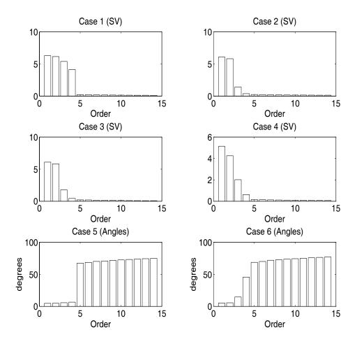
**Figure 5.4** The average singular values (Case 1-4) and angles (Case 5-6) that indicate the model order. For Case 1 and 5, the order is clearly equal to 4 (this is expected, since the data was generated by a fourth order system). For Case 2,3,4 and 6, the order is less clear. This is not unexpected, since one of the dynamic modes is filtered out by introducing either  $W_{\rm low}(z)$  or  $W_{\rm high}(z)$ .
