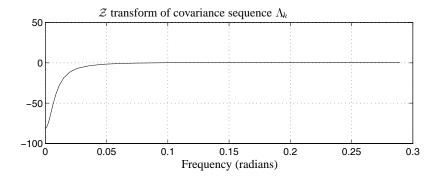
**Figure 3.15**  $\mathbb{Z}$ -transform of one of the identified "non-positive" covariance sequences (see (3.32)). When the covariance sequence would be positive real, its  $\mathbb{Z}$ -transform would have been positive. This Figure indicates the severe violation of the positivity constraint for some of the identified sequences.
