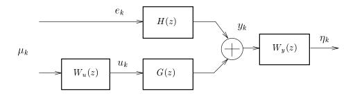
**Figure 5.1** Cascade system used for the interpretation of frequency weighted balancing. The weights  $W_u(z)$  and  $W_y(z)$  are user defined. Note that the noise input  $e_k$  has no extra weight, since from an input-output point of view, this weight is indistinguishable from H(z).
