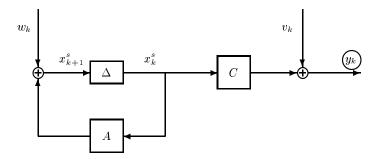
Figure 3.2 A linear time-invariant stochastic system with outputs  $y_k$  and states  $x_s^s$ , described by the matrices A, C and the covariance matrices Q, S, R. The symbol  $\Delta$  represents a delay. In the stochastic identification problem, only the output is measured. The state is unknown, but will be determined as an intermediate result of the subspace identification algorithms.
