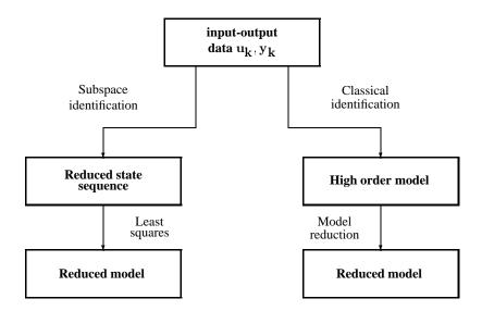
**Figure 1.6** System identification aims at constructing state space models from input-output data. When a reduced order model is required, in some classical approaches (to the right), one first identifies a high order model and then applies a model reduction technique to obtain a low order model. The left hand side shows the subspace identification approach: Here, we first obtains a "reduced" state sequence, after which one can identify directly a low order model.
