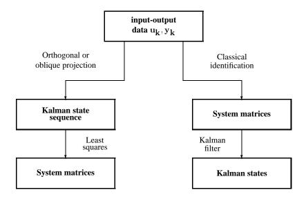
**Figure 1.5** System identification aims at constructing state space models from input-output data. The left hand side shows the subspace identification approach: first the (Kalman filter) states are estimated directly from input-output data, then the system matrices can be obtained. The right hand side is the classical approach: first obtain the system matrices, then estimate the states.
