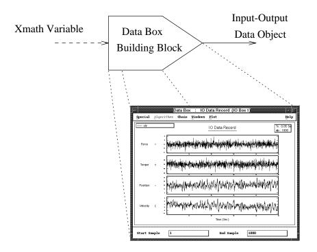
**Figure 6.4** An example of a data box. The input of the data box is an Xmath variable, the output is an **ISID** data object. Just as algorithms, data boxes have an algorithm window associated with it. This window allows for graphical interaction with the parameters.
