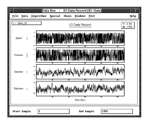
**Figure 6.8** Data set used for the identification of the glass tube production process. The inputs (top two signals) are drawing speed and mandrel pressure. They are excited using pseudo-binary noise sequences. The outputs (bottom two signals) are tube diameter and thickness.
