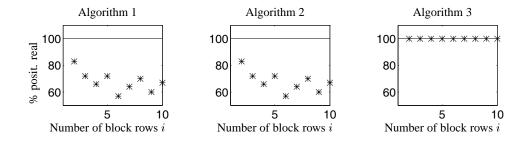
**Figure 3.16** Percentage identified positive real sequences for 100 Monte Carlo experiments, for a different system as in Figure 3.14. This Figure illustrates that for algorithm 1 and 2, the identified covariance sequence is *not* always positive real, even for larger i. This Figure was generated using the Matlab file sto sim3.m.
