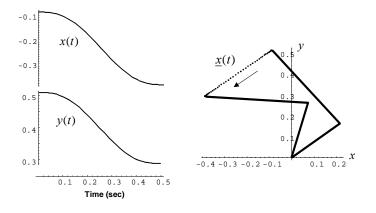
Figure 3. A minimum jerk motion in two dimensions is a straight line. The end-effector location of a two-link arm is moved from (-0.09, 0.51) to (-0.39, 0.29) in 0.5 seconds. The trajectory of x- and y- components of end-effector location are plotted, as well as end-effector location.
