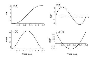
Figure 2. Minimum jerk trajectory. The function x(t) that has the minimum jerk cost function as it travels 10 cm over 0.5 seconds.
