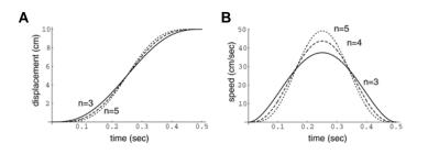
Figure 4. Movements with minimum jerk, snap, or crackle. A. A minimum jerk (n=3), a minimum snap (n=4), and a minimum crackle (n=5) trajectory. The variable n refers to the order of the derivative in Eq.(3). **B**. Speed of the movement for each trajectory. Note that the ratio of peak speed to average speed increases as n increases.
