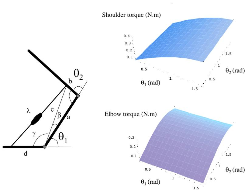
Figure 3. **A two-joint muscle.** The torque on the shoulder ( $\theta_1$ ) and elbow ( $\theta_2$ ) is plotted as a function of angle of each joint for a constant muscle force of 10 Newtons (N). Link lengths:  $a=0.33$ ,  $d=0.04$ ,  $b=0.03m$ .
