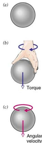
*Figure.1. Angular velocity and torque. A quick twist of the wrist imposes a torque on the ball that results in the ball acquiring angular velocity. The angular velocity vector is directed along the axis of rotation. Its direction is the same as that of the torque vector. (From L. A. Bloomfield, “How things work: The physics of everyday life”, Wiley, 2001).*
