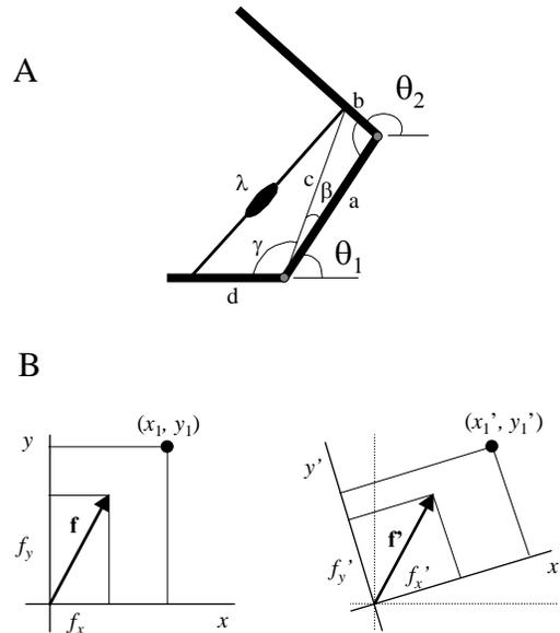
**Figure 4. A. A two joint muscle acting on a two-link system.** The system is identical to Figure 3 except that the angle of the second link is measured with respect to an absolute axis, rather than relative to the angle of the first link. **B. Rotation of a coordinate system in which the position of a point is described**
